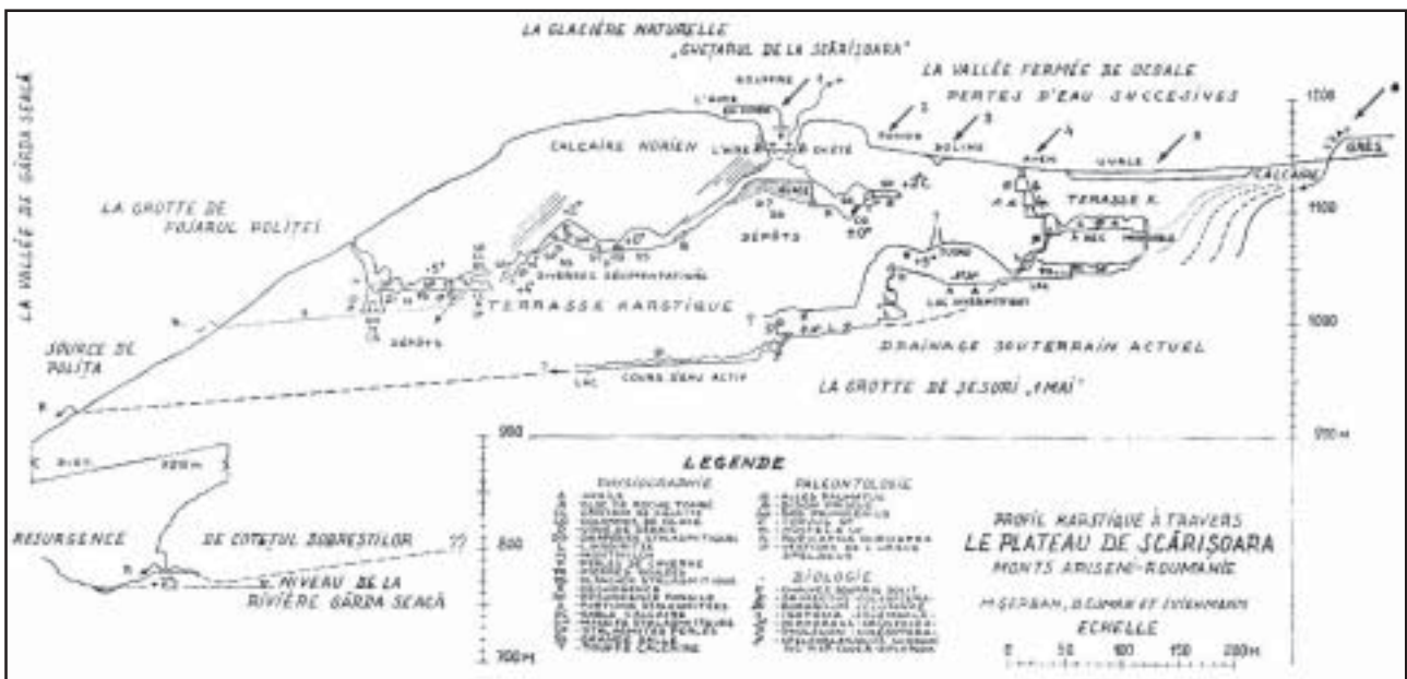
Figure 1.9. Karst cross-section across Scărișoara plateau (after M. ȘERBAN et al., 1957).
