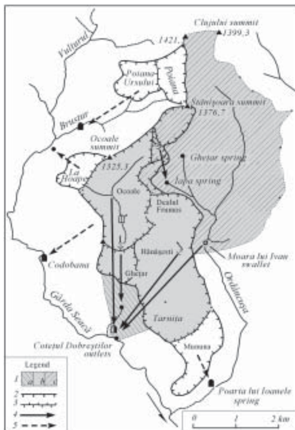
Figure 3.5. The Cotețul Dobreștilor karst system. Legend: 1 - Extension of the karst system: a - Karstic slope basin; b - Internal drainage area; c - Diffuence surface; 2 - Boundary of internal drainage area; 3 - Boundary inside internal drainage areas; 4 - Proven groundwater flow connexion; 5 - Inferred groundwater flow connexion.
