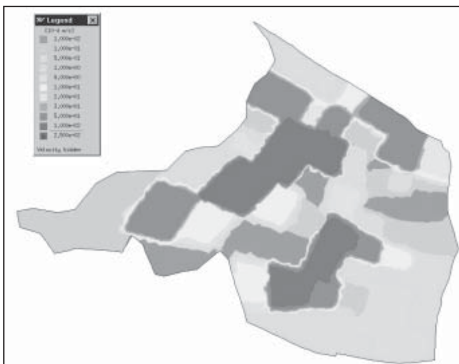
Figure 8. Calibration of horizontal conductivity for deep aquifer.
